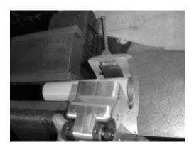
3. Start cutting by slowly pressing on Power Switch to make CH to rotate around tube. Rotate CH slowly for first turn to allow blade to make first complete cut grove. Do not force tool. Let tool align itself on the tube to get square cut. Forcing tool out of square plane can damage blade and result in out of square cut.
