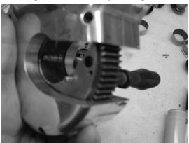
new blade and push pin back trough larger hole. Check that blade moves free under spring return when pressed by finger. Screw back setscrew to cover pin pass hole.
